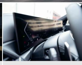
The all-new BMW Curved Display – combining a 12.3" Digital Instrument Cluster and 14.9" Central Information Display – makes interacting with the latest iDrive 8 Operating System easy. Surround yourself with advanced BMW driving technology. The new 3 Series includes even more convenient features such as Active cruise control with Stop&Go function that will make your journey even more enjoyable and safer.
