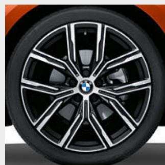
□ 19" light alloy wheels Y-spoke style 783 Bicolour Jet Black with mixed tyres and run-flat tyres, gloss-lathed, wheel size front 8J x 19 with 225/40 R19 tyres, wheel size rear 8.5J x 19 with 255/35 R19 tyres.*
