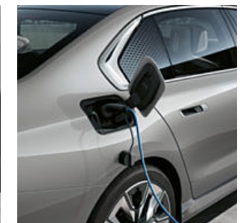
The fast charging cable (mode 3) allows you to charge the high-voltage battery at public charging stations – 3-phase and with a charging capacity of up to 11kW.
