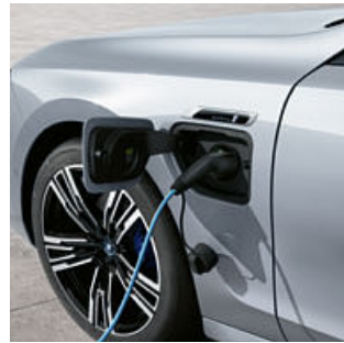
The fast charging cable (mode 3) allows you to charge the high-voltage battery at public charging stations – 3-phase and with a charging capacity of up to 11kW.
